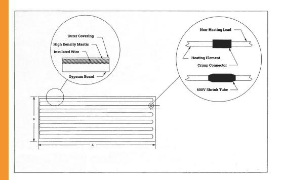
Cutaway view of a Radiant Ceiling Heating Panel
