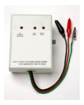
1. Take the red clip and connect it to the bare wire of the white lead wire. Do the same connecting the black clip to the black lead wire. Connect the green clip to the steel braid (see diagram). Turn S.I.D. on. If there are no lights or buzzing then the cable is good. Turn S.I.D. off and disconnect so that you can install the floor warming system.
